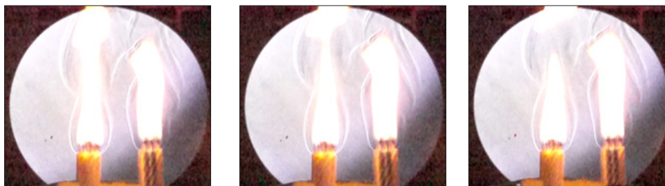
Figure 12. Different stages of flame puffing, N = 7, r = 3.6 cm
