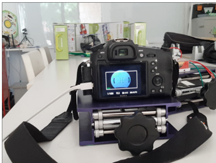
Figure 6. The schlieren setup
